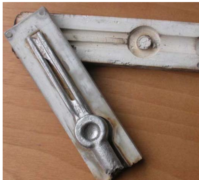
Figure 7 Photograph of a mechanical part obtained by aluminium casting in a ceramic green mould.
